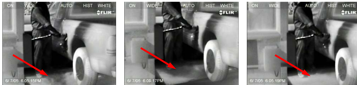
Figures 4A, 4B, 4C. Gasoline fumes seen by the GasFindIR accumulating near the pavement, then dissipated by a breeze.
