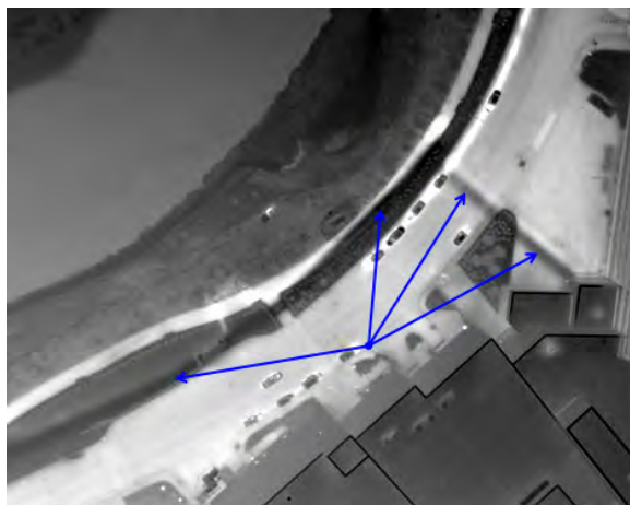
Figure 5. Buried chilled water line cools the surface above the line.
