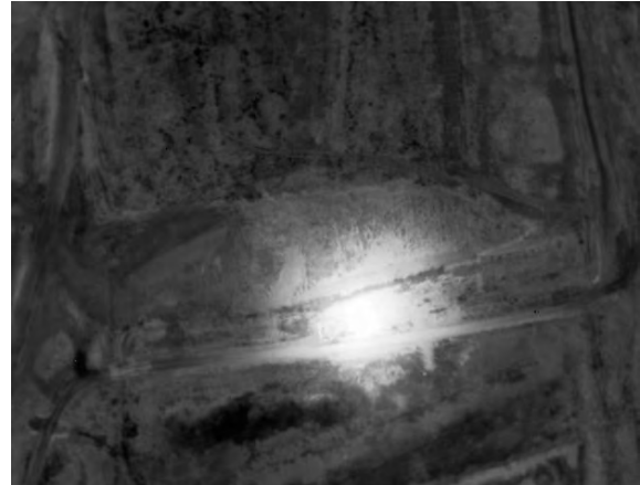
Figure 9. IR imagery of a subsurface fire in landfill.
