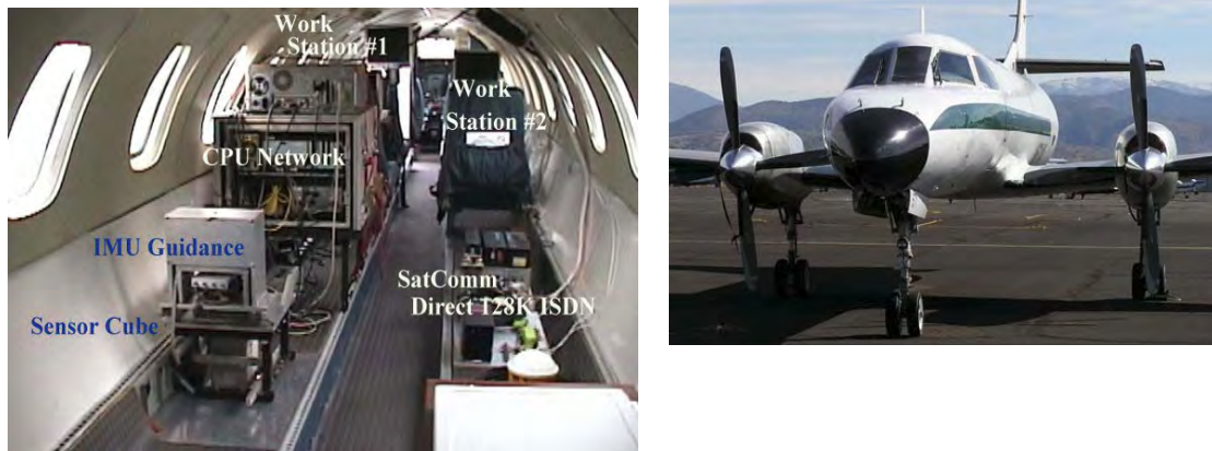
Figure 2. High resolution aerial IR imaging, data collection system, and aircraft.
