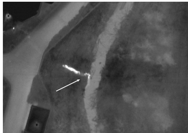
Figure 6. IR Imagery of a storm water drainage system outfall flowing into a creek.
