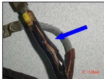
Figure 6: Photos show the damaged cable after installation of a new one
