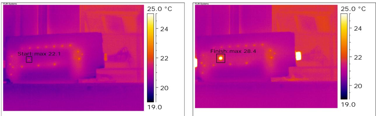
Figure 3. Initial (left) and final (right) infrared thermograms of wall board screws in and near an ABS vent pipe.
