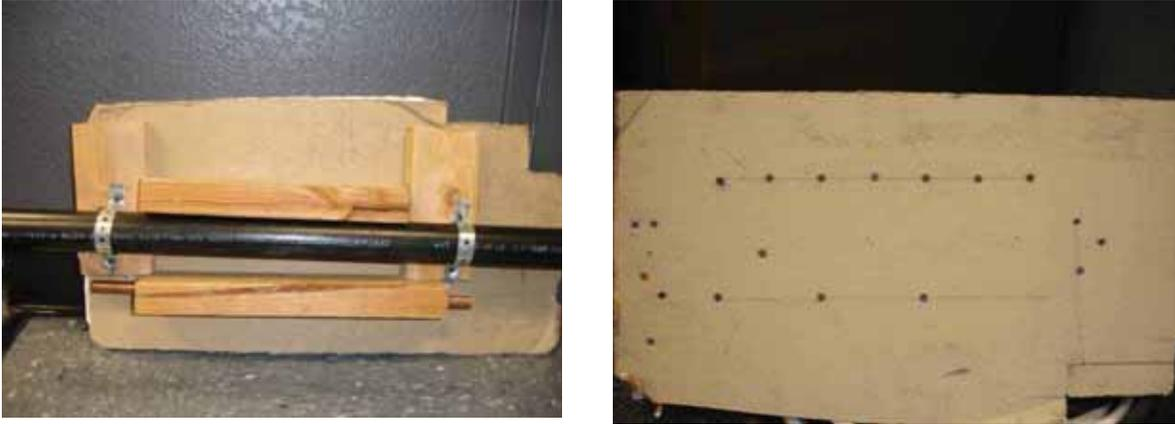
Figure 2. The back and front of a test jig for screw-into-pipe defects.
