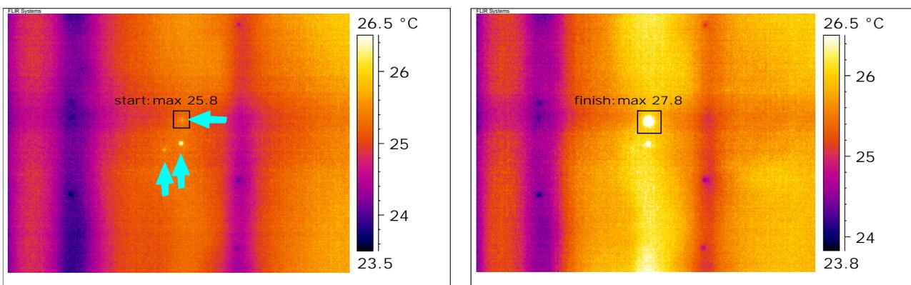
*Figure 6. Initial (left) and final (right) thermograms of wall board screws in and near an ABS vent pipe.*
