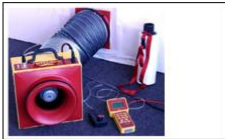
Figure 13a. Duct testing equipment: Image courtesy of Retrotec
