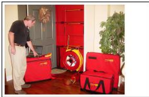
Figure 7a. Door-Fan Testing
